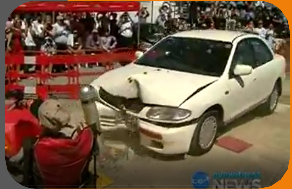
Televised actual crash testing of Energy Absorbing Bollards
