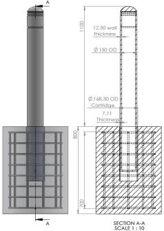
The Armour Security Bollard (ASB) is capable of stopping a 1800kg vehicle @ 60kph.
