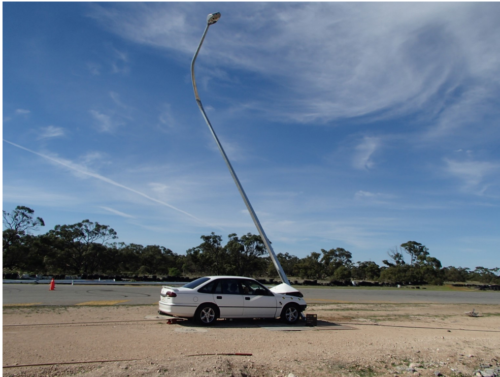
EASLP test photo. A car travelling at 60kph has been arrested by the Energy Absorbing Light Pole and is supporting the EASLP against the vehicle.
