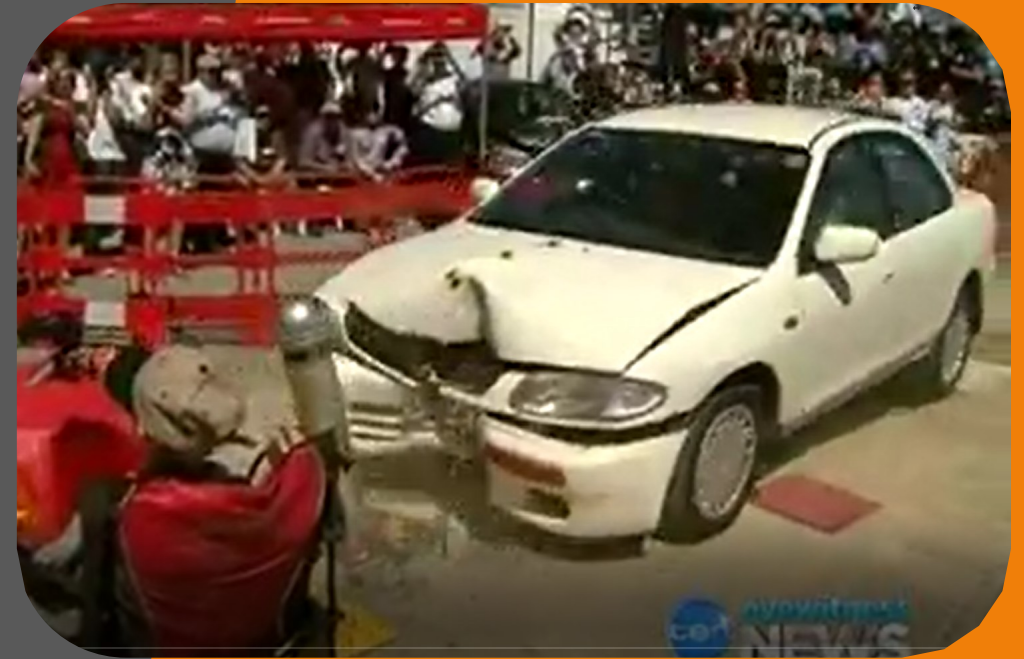
Televised crash testing of Energy Absorbing Bollards
