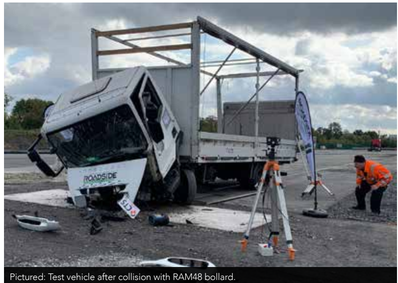
Pictured: Test vehicle after collision with RAM48 bollard.
